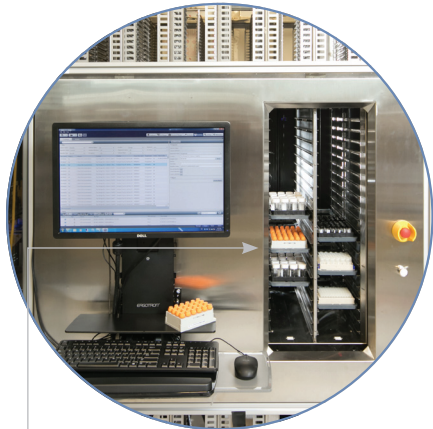
Introduce and retrieve samples using the Input/Output station and the "3-click" software.
