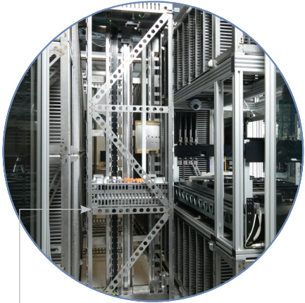
Tray shuttle robot to move the samples to the storage locations and tube picker inside Verso.
