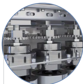
Our patented external magnetic couplers drive the internal robotics.
